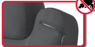
Seat belt opening custom formed
